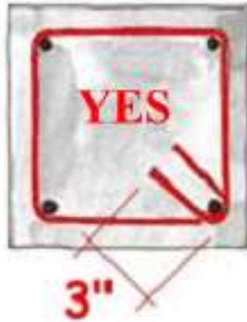
Fig 08: Hooks of column and beam at 135 degree and length of hook is 3inches/7.5 cm.
